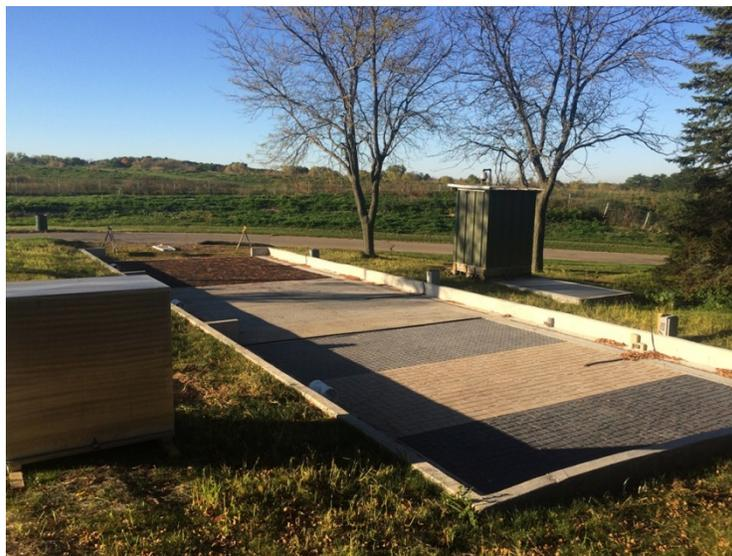
From left to right, the testing area includes permeable asphalt, permeable concrete and permeable pavers, all installed at the end of a campus parking lot. All three of these surfaces contain tiny holes or channels within them that allow liquids like rain and
